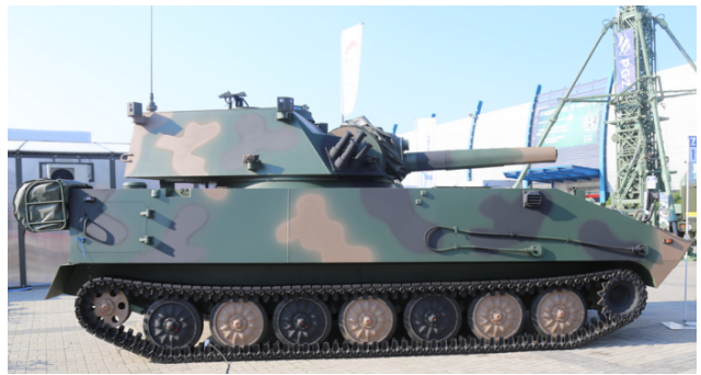
Figure 2. SOD Situational Awareness System mounted on a self-propelled 120mm RAK mortar.
